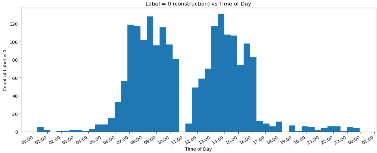
Figure 3. Distribution of construction noise events across the 24-hour data collection period (Nov 12th, 2025, 11:30 am - Nov 13, 2025) grouped into half-hour intervals. Indications of high construction activity are evident throughout the morning and afternoon consistent with standard work hours.
